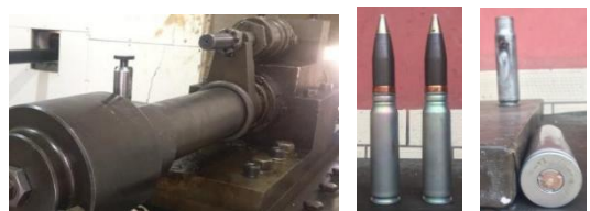
图9 膛压强度试验设备 Fig.9 Chamber pressure strength test equipment
