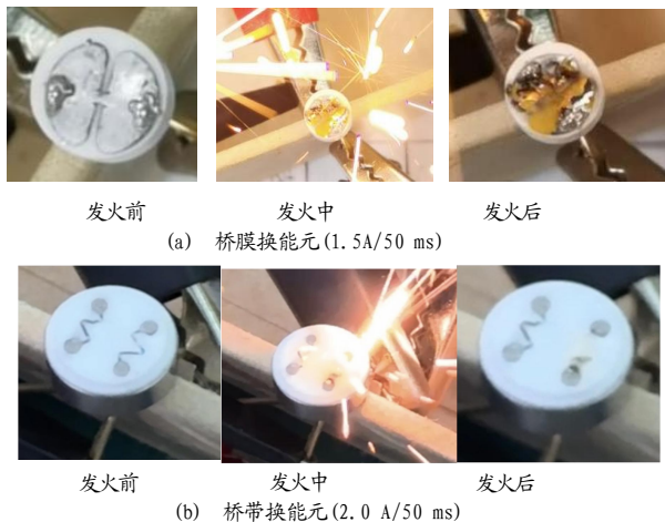
图8 50 ms 脉冲恒流爆发试验的换能元照片 Fig.8 Photographs of transducer during 50 ms pulse constant current burst test
