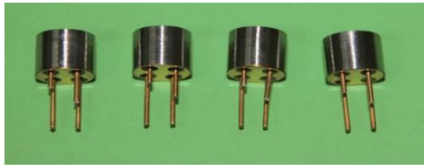
图12 集成平面三电极开关的冲击片雷管实物图 Fig.12 Physical diagram of exploding foil initiator with integrated planar three-electrode switch
