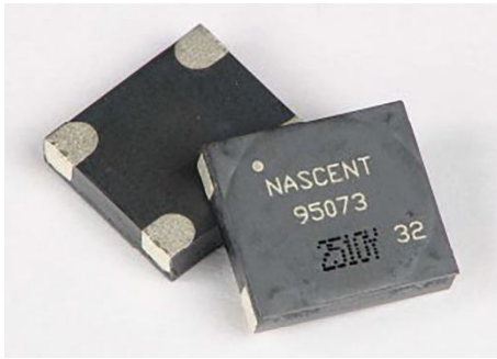
图3 美海军引信第64届年会公开报道的LTCC变压器 Fig.3 LTCC transformer reported at the 64th Fuze Annual Conference
