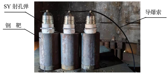
图8 SY射孔弹穿深试验示意图 Fig.8 Diagram of steel plate test of SY shaped charge
