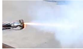
图5 余火点燃相邻点火管 Fig.5 Residual fire igniting adjacent ignition tube
