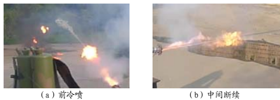
图6 点射时出现前冷喷和中间断续现象 Fig.6 The phenomenon of front cold spray and middle intermittent appears during point injection
