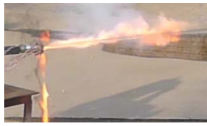
图4 余火点燃余油 Fig.4 Residual oil ignited by residual fire
