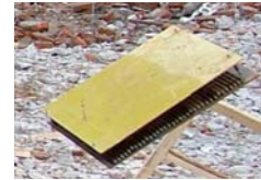
图 5 油路管道冲击引燃等效靶照片 Fig.5 Photo of the equivalent target of the fuel pipelines used for the impact inflame damage experiment
