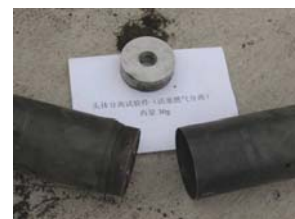
图6 分离后的第5发试验件(30g药量) Fig.6 The fifth specimen (with 30g powder) after separation process
